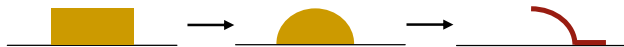
Fig. 13 Transition of a rectangular section of photo resist to a curved section of photoresist to a curved metal structures
